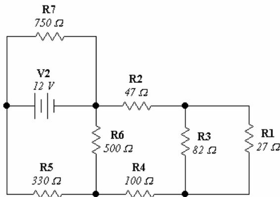
Soluciones corrientes:  $I_{R_1} = 14.88_{[mA]}$ ;  $I_{R_2} = 19.78_{[mA]}$ ;  $I_{R_3} = 4.90_{[mA]}$ ;  $I_{R_4} = 19.70_{[mA]}$ ;  $I_{R_5} = 26.33_{[mA]}$ ;  $I_{R_6} = 6.62_{[mA]}$ ;
