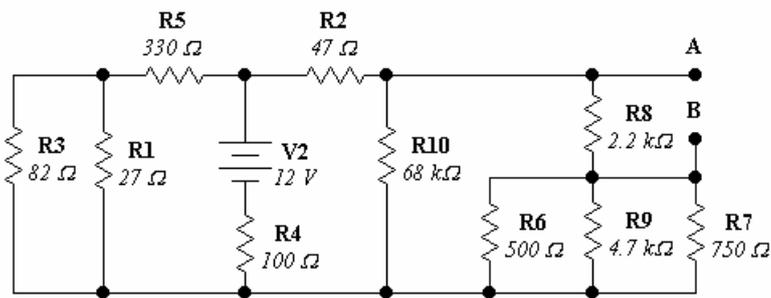
Solución:  $I_{R_1} = 19.42_{[mA]}$ ;  $I_{R_2} = 3.70_{[mA]}$ ;  $I_{R_3} = 6.39_{[mA]}$ ;  $I_{R_4} = 29.53_{[mA]}$ ;  $I_{R_5} = 25.82_{[mA]}$ ;  $I_{R_6} = 2_{[mA]}$ ;  $I_{R_7} = 1.33_{[mA]}$
