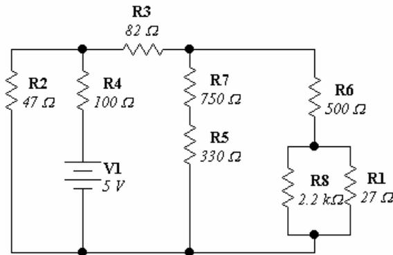
Solución corrientes:  $I_{R_1} = 2.26_{[mA]}$ ;  $I_{R_2} = 31.68_{[mA]}$ ;  $I_{R_3} = 3.41_{[mA]}$ ;  $I_{R_4} = 35.10_{[mA]}$ ;  $I_{R_5} = 1.11_{[mA]}$ ;  $I_{R_6} = 2.29_{[mA]}$ ;  $I_{R_7} = 1.11_{[mA]}$ ;  $I_{R_8} = 27.76_{[\mu A]}$
