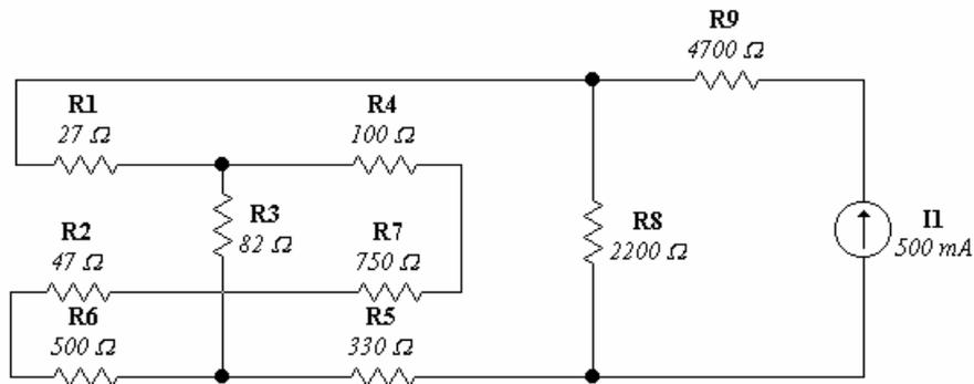
Solución corrientes:  $I_{R_1} = 417.54_{[mA]}$ ;  $I_{R_2} = 23.14_{[mA]}$ ;  $I_{R_3} = 394.39_{[mA]}$ ;  $I_{R_4} = 23.14_{[mA]}$ ;  $I_{R_5} = 417.54_{[mA]}$
