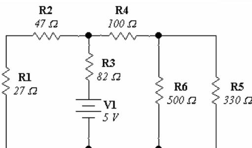
Solución corrientes:  $I_{R_1} = I_{R_2} = 28.35_{[mA]}$ ;  $I_{R_3} = 35.38_{[mA]}$ ;  $I_{R_4} = 7.02_{[mA]}$ ;  $I_{R_5} = 4.22_{[mA]}$ ;  $I_{R_6} = 2.79_{[mA]}$ .
