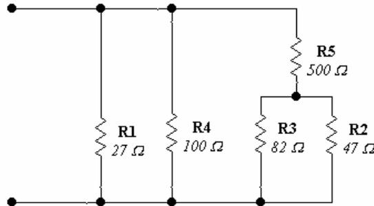
Solución:  $I_{[R_1]} = 2.97_{[A]}$ ;  $I_{[R_2]} = 141.76_{[mA]}$ ;  $I_{[R_3]} = 81.25_{[mA]}$ ;  $I_{[R_4]} = 802.81_{[mA]}$ ;  $I_{[R_5]} = 223.02_{[mA]}$
