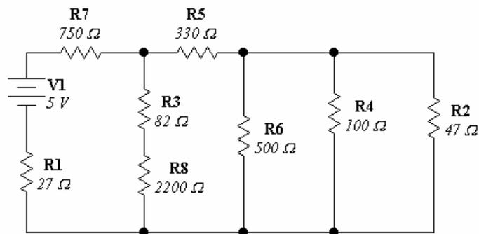
Solución corrientes:  $I_{R_1} = I_{R_7} = 2.12_{[mA]}$ ;  $I_{R_2} = 420.85_{[\mu A]}$ ;  $I_{R_3} = I_{R_8} = 1.46_{[mA]}$ ;  $I_{R_4} = 197.8_{[\mu A]}$ ;  $I_{R_5} = I_{R_6} = 658.92_{[\mu A]}$ ;  $I_{R_8} = 39.56_{[\mu A]}$
