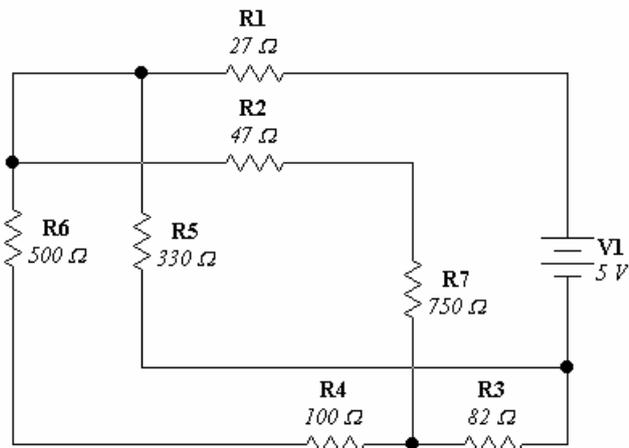
Solución corrientes:  $I_{R_1} = 23.51_{[mA]}$ ;  $I_{R_2} = I_{R_7} = 4.41_{[mA]}$ ;  $I_{R_3} = 10.29_{[mA]}$ ;  $I_{R_4} = I_{R_6} = 5.88_{[mA]}$ ;  $I_{R_5} = 13.22_{[mA]}$
