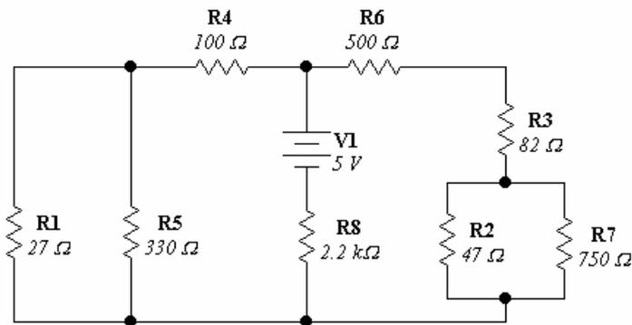
Soluciones corrientes:  $I_{R_1} = 1.66_{[mA]}$ ;  $I_{R_2} = 338.10_{[\mu A]}$ ;  $I_{R_3} = I_{R_6} = 359.29_{[\mu A]}$ ;  $I_{R_4} = 1.80_{[mA]}$ ;  $I_{R_5} = 136.13_{[\mu A]}$
