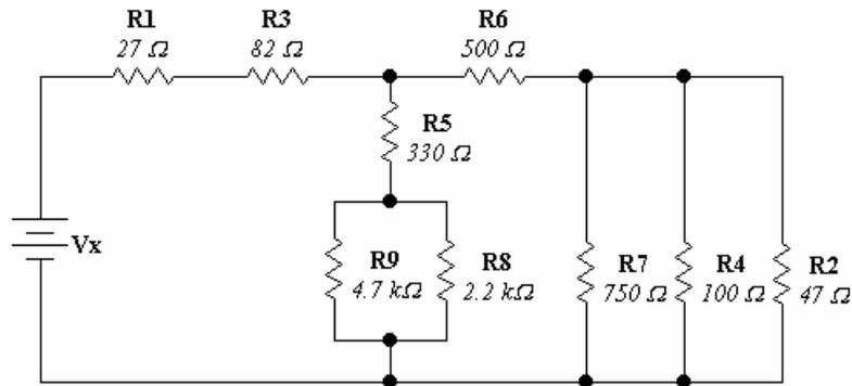
Solución:  $V_x = 13.88_{[V]}$ ;  $V_{[R_1]} = 720.63_{[mV]}$ ;  $V_{[R_2]} = V_{[R_4]} = V_{[R_7]} = 640_{[mV]}$ ;  $V_{[R_3]} = 2.18_{[V]}$ ;  $V_{[R_5]} = 1.98_{[V]}$ ;  $V_{[R_6]} = 10.34_{[V]}$ ;  $V_{[R_8]} = V_{[R_9]} = 9_{[V]}$
